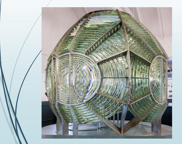
Because of its amazing efficiency, a Fresnel lens could easily throw its light 20 or more miles to the horizon. Lens designs resembled a giant glass beehive, with a light at the center. The Fresnel lens reduces the amount of material required compared to a conventional lens by dividing the lens into a set of concentric annular sections. An ideal Fresnel lens would have an infinite number of sections. In each section, the overall thickness is decreased compared to an equivalent simple lens.
